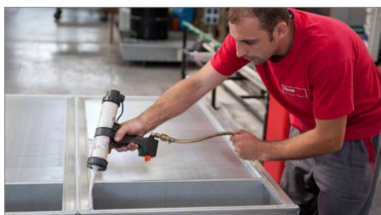
Fgi. 3: Apply sealing compound
