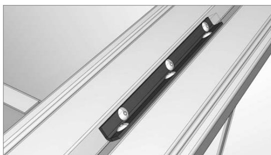
Fgi. 5: Rivet on the angle brackets
