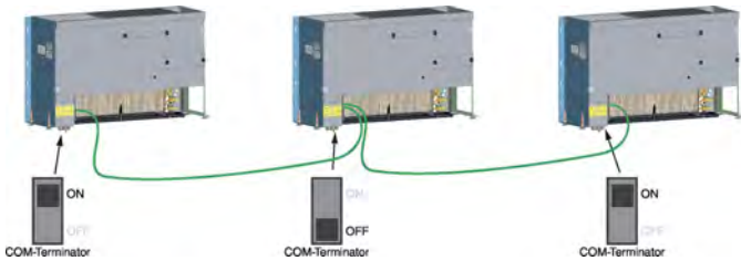
Fig. 15: FSL-CONTROL II communication of 3 units
