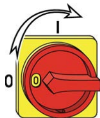
Fig. 38: Switching on the mains isolator
