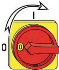
Fig. 39: Switching on the mains isolator
