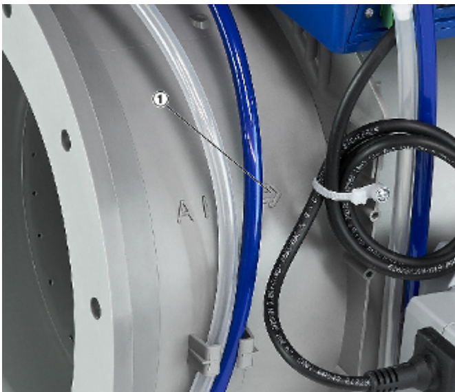
Fig. 9: Air direction arrow on the TVLK
