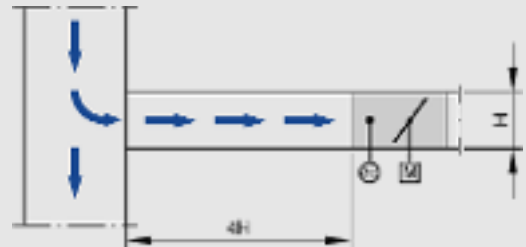
Fig. 17: Junction from a vertical main duct (view from the side)
